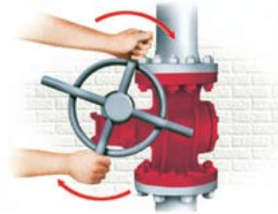
Turn the hand wheel in a clockwise direction until the valve is fully closed.
