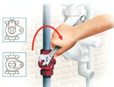
Turn the valve a quarter turn to the right or left , until both holes are aligned.
