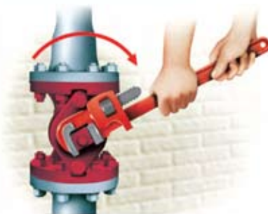
Turn the valve in a clockwise direction until it is fully closed.
